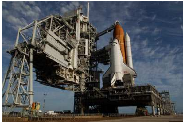
The rotating service structure is rolled back from around space shuttle Endeavour Monday morning.
